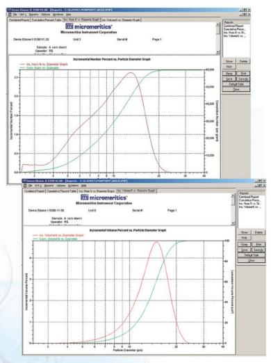
Volume and number distributions calculated for an analysis of a commercial cornstarch. The number distribution is comparable to a microscope analysis. The volume distribution is comparable to the results from the other particle size analyzers such as the Micromeritics SediGraph and Saturn DigiSizer, or that from sieve analysis. Note that the Elzone II produces directly a number-based distribution. The equivalent spherical volume distribution is calculated from the number distribution.
