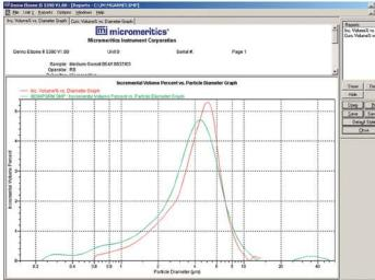
Overlay of cumulative volume percent finer than diameter and volume frequency, for a medium garnet abrasive powder, analyzed with the Elzone II and the Micromeritics SediGraph. The Elzone II reporting system can report size distributions determined using other Micromeritics particle size analysis instruments such as the SediGraph and Saturn DigiSizer.
