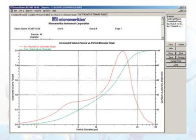
Complete analysis of broadly dispersed chocolate sample, a mixture of cocoa powder, sugar, and milk solids. Analysis data from three orifice tubes are merged together automatically by the Elzone II software.
